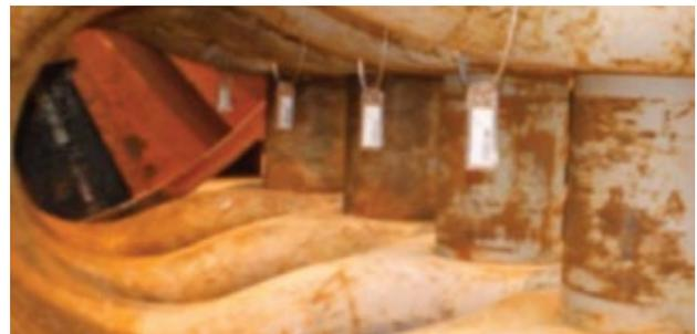
The tags are so strong that if pulled it is the metal fixing on the trolley that will often break off before the tag breaks (the average tensile strength of the tags is 120kg+).
